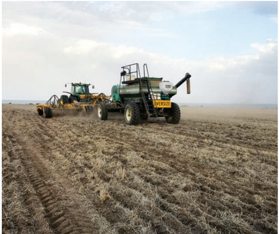
A CHANGE IN DISC CONFIGURATION AND ROW SPACING PLUS THE ABILITY TO DELIVER LIQUID NUTRIENTS HAS IMPROVED SEEDING-TIME PERFORMANCE, WEED CONTROL AND CROP HEALTH AND PERFORMANCE.
