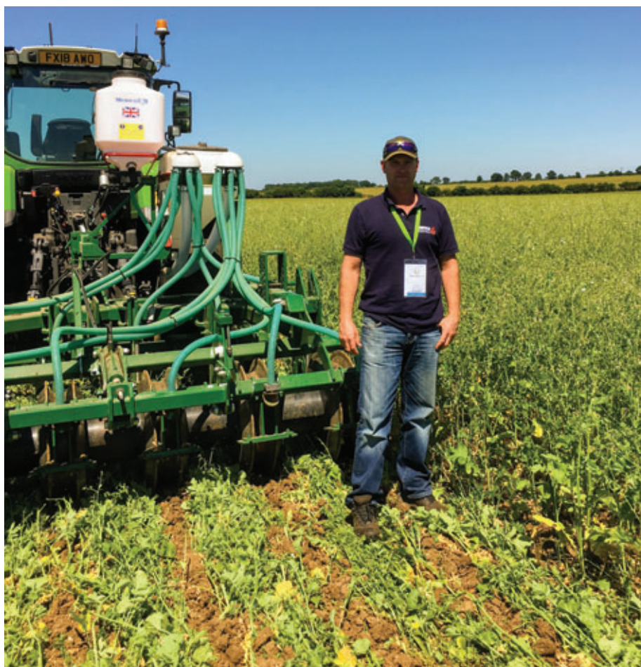
DURING HIS OVERSEAS STUDY TOUR, GRANT HAD AN OPPORTUNITY TO CHECK OUT THIS MACHINE, WHICH ROLLS STANDING VEGETATION ONTO THE SOIL AND SOWS A FOLLOWING CROP IN A SINGLE PASS.
