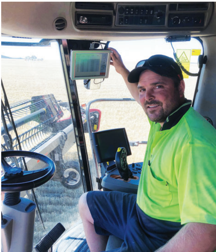
SHANE JERICHO, AT THE CONTROLS OF THE FAMILY’S HEADER, ADJUSTS THE SCREEN OF THE GRAIN ANALYSER, WHICH RECORDS THE AVERAGE PROTEIN LEVEL OF EACH HEADER BIN OF GRAIN. THE HEADER DRIVER IS RESPONSIBLE FOR COMMUNICATING THAT PROTEIN LEVEL, WHICH DETERMINES WHICH FIELD BIN THE GRAIN IS TO GO INTO, TO THE CHASER BIN DRIVER.
