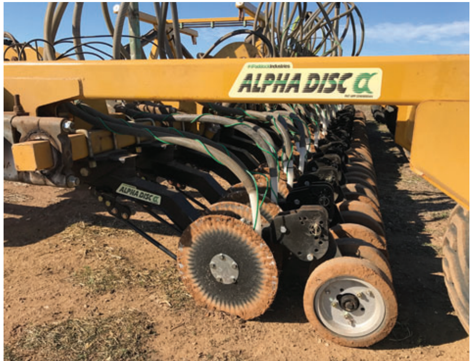
JASON IS FINDING THAT THE SOIL THROW FROM HIS ALPHA DISCS, COMBINED WITH CLOSER ROWS, HAS IMPROVED THE EFFICACY OF HIS PRE-EMERGENCE HERBICIDES, WHICH HAS GIVEN HIM THE CONFIDENCE TO USE MORE EXPENSIVE CHEMISTRY.
