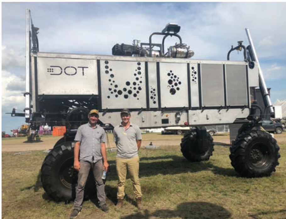
BOYD CARTER AND FELLOW NUFFIELD SCHOLAR DYLAN HIRSCH ARE DWARFED BY THIS AUTONOMOUS VEHICLE, TECHNICALLY A DOT 'IMPLEMENT CARRIER' DESIGNED TO BE FITTED WITH 'TOOLS' TO UNDERTAKE DIFFERENT FARMING TASKS, THEY ENCOUNTERED IN SASKATCHEWAN, CANADA, DURING THEIR NUFFIELD STUDY TOURS.
